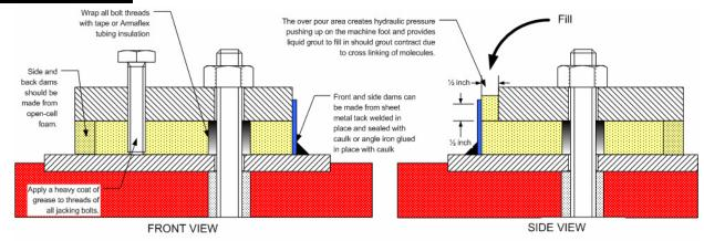
Using open-cell foam damming material, build a dam around 3 sides of the area to be chocked. Wrap the anchor bolt with tape so the Chockfast will not stick to it, Install a metal dam along the front of the chock approximately ½" to ¾" (12mm to 18mm) from the mounting flange. Seal the flange with strip caulking, or Silicone to prevent leaks. Install foam in the overpour area to the top of the mounting flange to prevent the Chockfast from leaking.
